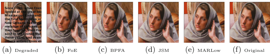
Fig. 8. Visual quality comparison of text removal for image Barbara and Parthenon . (a) The degraded image with text mask; (b) – (e) Restoration results by FoE, BPFA, JSM, and the proposed method. (f) The ground truth image.
